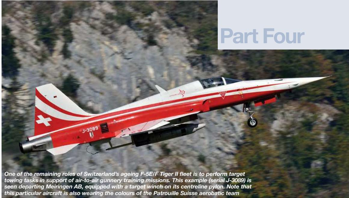
One of the remaining roles of Switzerland's ageing F-5E/F Tiger II fleet is to perform target towing tasks in support of air-to-air gunnery training missions. This example (serial J-3089) is seen departing Meiringen AB, equipped with a target winch on its centreline pylon. Note that this particular aircraft is also wearing the colours of the Patrouille Suisse aerobatic team
